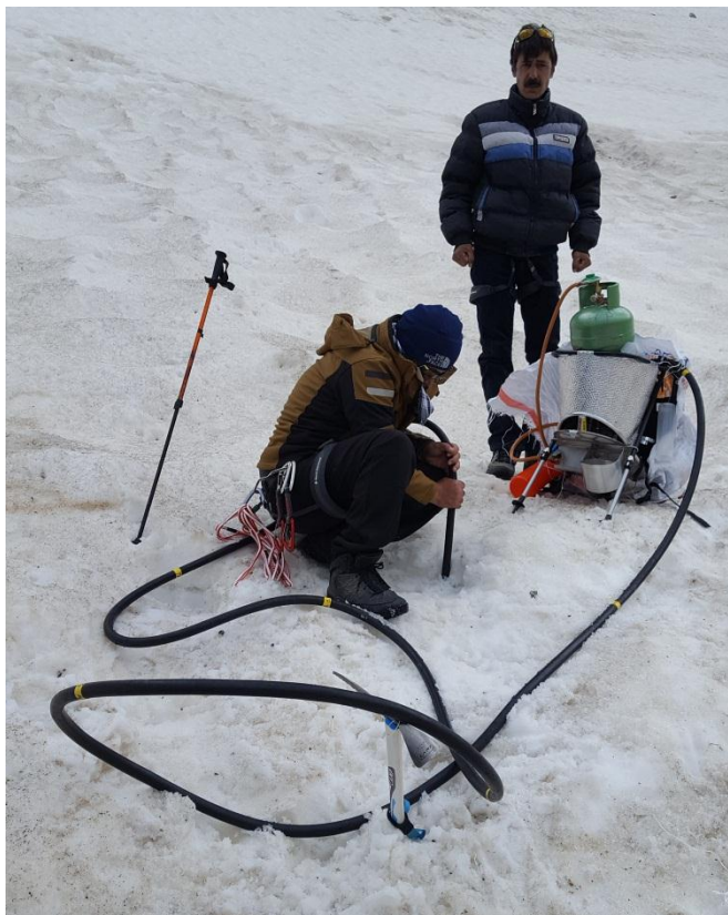
Fig-2 Drilling for installing the measurements sticks Using Heucke Ice Drill
